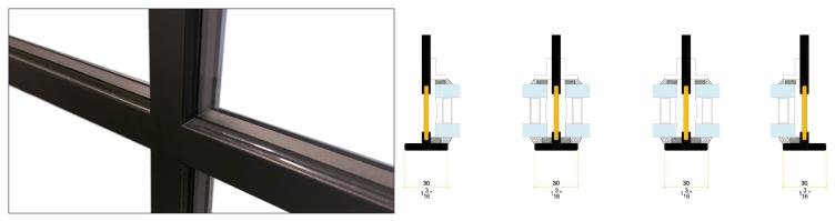
The traditional way to divide a large window is to divide it into smaller areas. Each surface contains its own piece of glass. All MHB glass stops fit into this system, including elastic putty seal.
